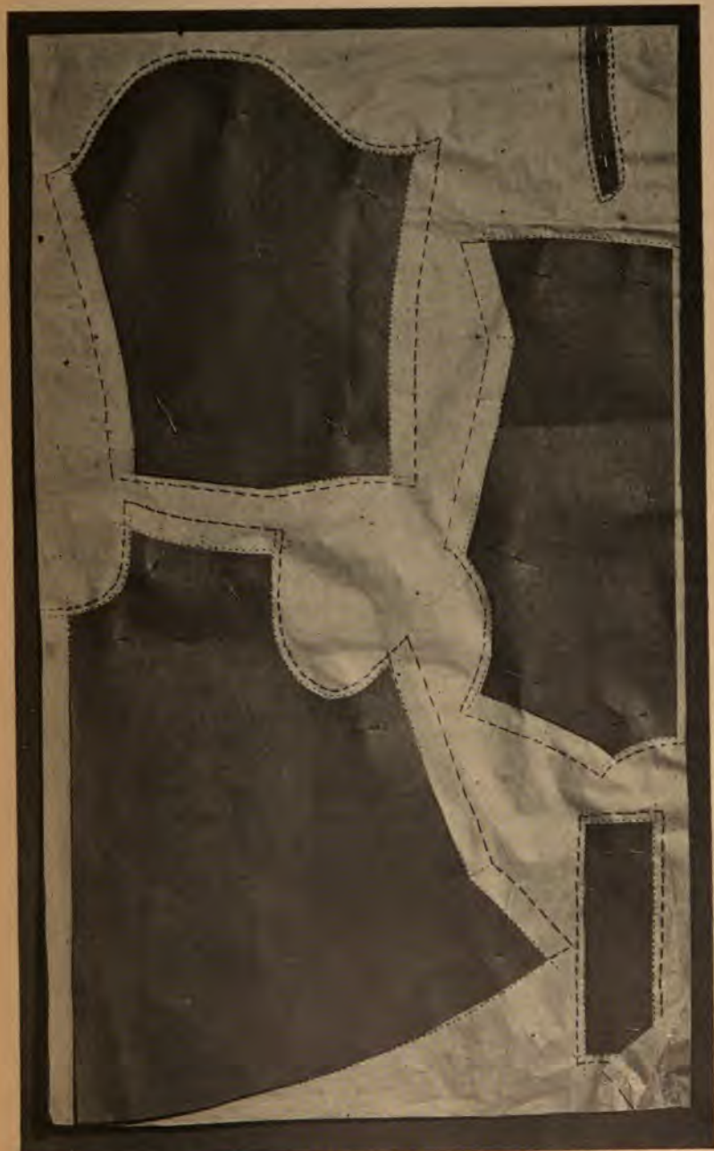
FIG. 38—Shirtwaist pattern placed on cambric or muslin, ready for cutting a trial waist.
